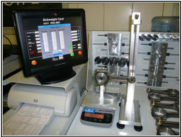
With this type of setup the weight values are directly sent to the computer software that allows the operator to log-in the weight of the part plus add the part number and description for later recall.
