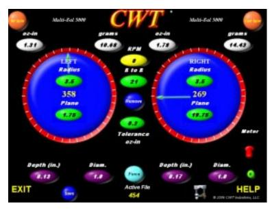
This particular example shows the left side unbalance @ 1.31 Oz-in and the right side @ 1.78 Oz-in. It also is telling the operator to remove 10.68 grams of weight from the outside edge of the crankshaft or if you decide to drill then by using a 1" drill you will need to drill .130 of an inch at the TDC Point.
