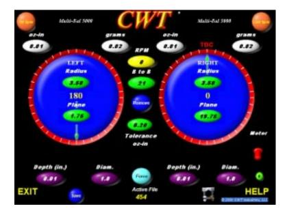
Notice that the magnitude of unbalance force has been reduced to 0.01 for both sides and that the position of any residual unbalance is equally opposed from the right and left side (180 degree). This crankshaft assembly is correctly balanced.
