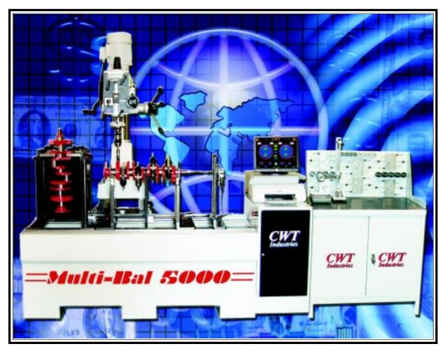
It takes about 20 seconds for the machine to determine both the position and magnitude of unbalance and display the data for the technician.
